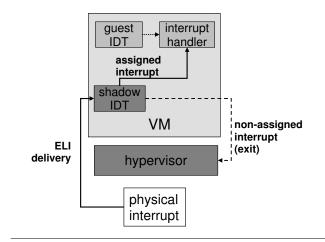
Figure 2. ELI interrupt delivery flow
